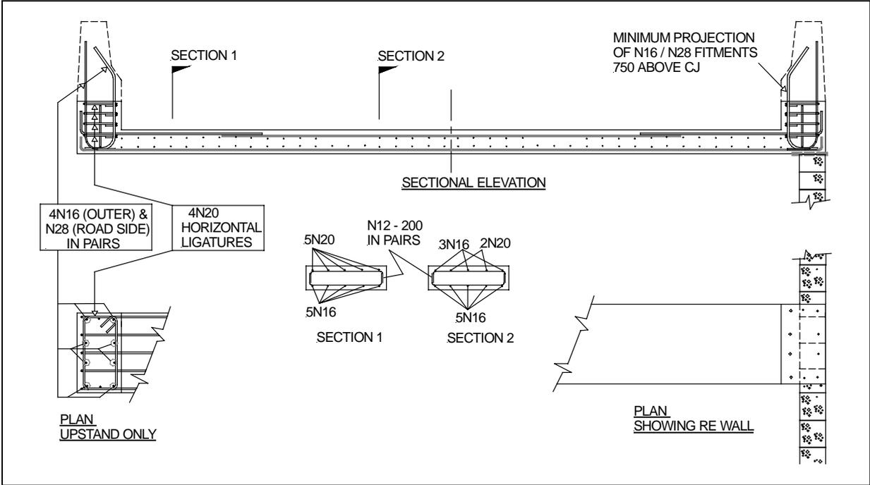
**Figure 6: Footing Reinforcing Liverpool Parramatta Bus Transitway**
