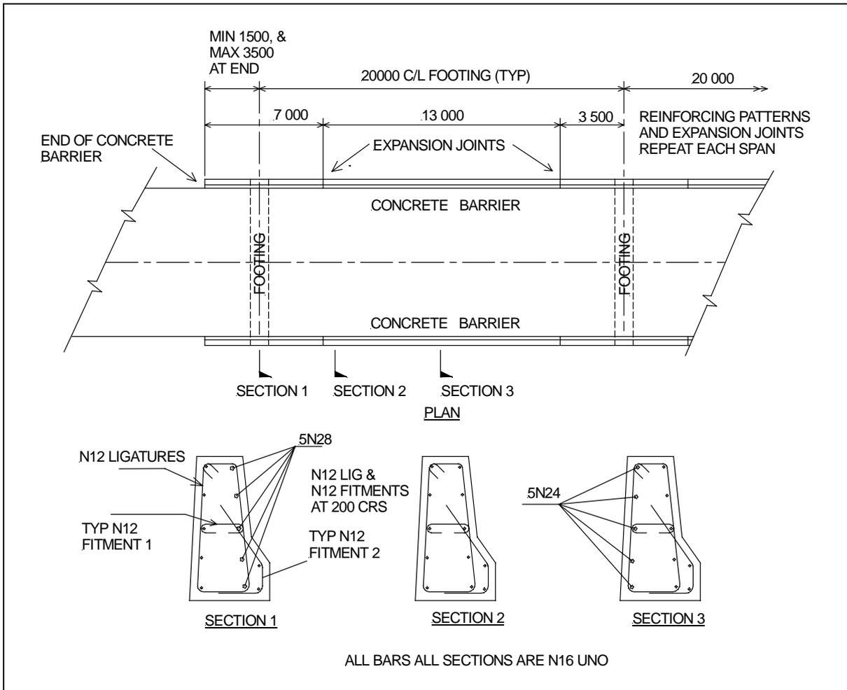
**Figure 4: Barrier Reinforcing Details - Liverpool Parramatta Bus Transitway**
