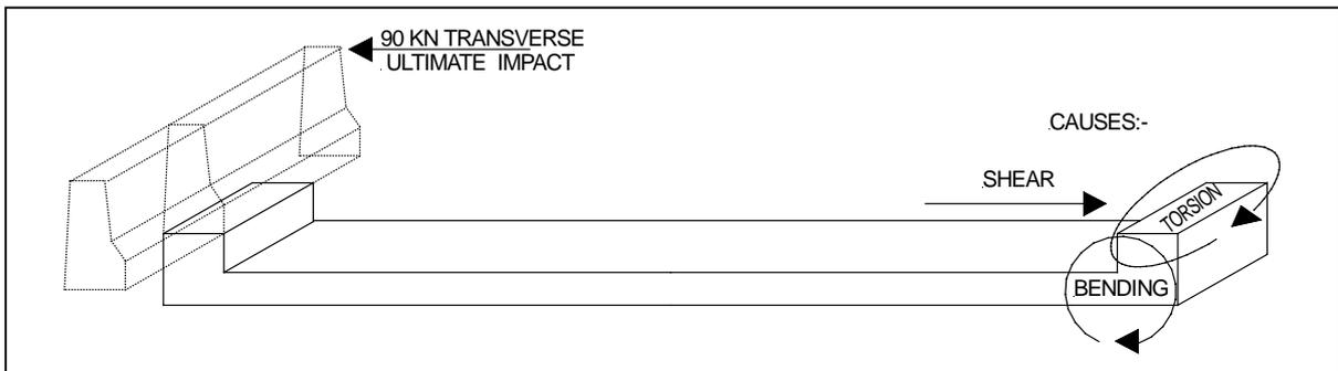
**Figure 5: Diagrammatic Isolated Footing Loads for Impact Barrier**
